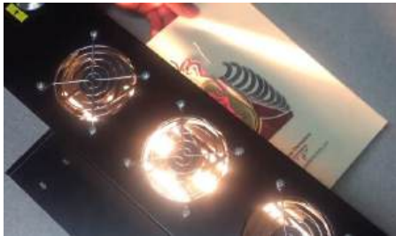
The swelling machine heats the paper and causes the inked areas to swell.
