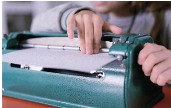
A Perkins braille is a typewriter used to emboss braille into paper.
