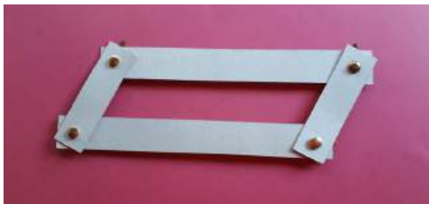
Foldable parallelograms made from laser-cut stainless steel (top left), Meccano (right) and card and split pins (bottom left).
