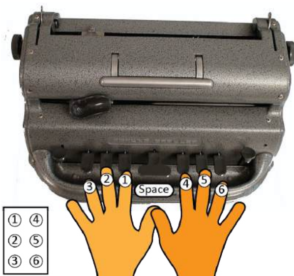
Perkins brailier. Combinations of six of the keys create the braille patterns.
